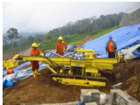
Seismic shot hole drilling for PT. Schlumberger Geophysics Nusantara at Kondur Site, Riau
