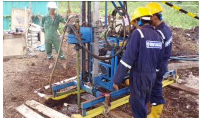
Seismic shot hole drilling for PT. Schlumberger Geophysics Nusantara at Kondur Site, Riau
